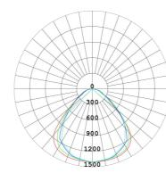
Wide light distribution means uniform light on wall ceiling and floors. Retrofit and new design may allow to reduce number of fittings overall. LGP™ - Light Guide Pattern technology, PMMA acrylic plate
